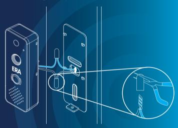
Step 1: Twist together the two wires, and then push the wires into the short end of the connector.
