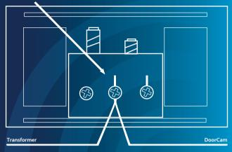
Result 1: Blue LED is ON for 5 seconds, and then red LED is ON for around 30 seconds. Finally the red and green LED will flash. This means the doorbell is working correctly. You can go to 'SETUP OPERATION'.
